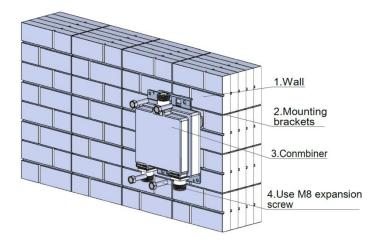
③ Whether it's pole or wall mounted , when installing the combiner, ANT output port facing up (Connected to antenna feeder), Input port facing down, connected to each signal source.
