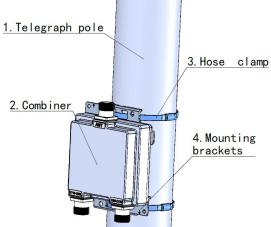
② For wall mounted installation, no hose clamp required. A number of screws are required to pass through the reserved hole in the bracket. Fasten the product firmly to the wall;
